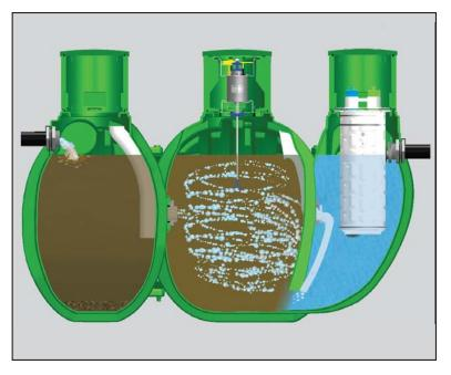
chamber hydraulic currents shall enter the sludge return and be directed through the Bio-Static device into the second zone of the clarification chamber. The Bio-Static sludge return shall accomplish resuspension and return of settled solids without disturbing the clarified liquid in the final settling zone and outlet zone.
